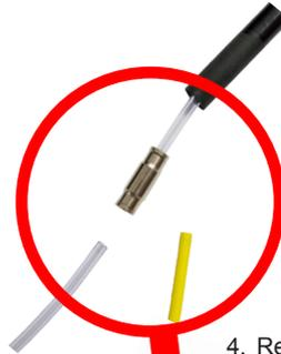
4. Remove the yellow plug from the push fit connector. Store in carry case pocket to be re fitted after use, this prevents moisture entering tubes when not in use, reducing likely-hood of blockage.
